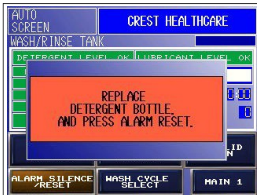
Figure 3-1. Typical Alarm Screen
