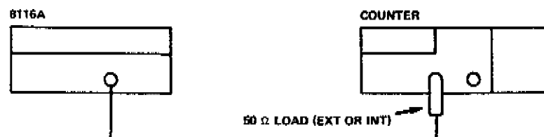
Figure 4-14. Test setup for Duty Cycle
