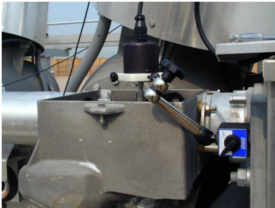
Rotary Transducer on Alstom HE 1014 Circuit Breaker
