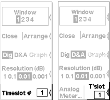
Fig. 4-28 Windows menu, softkey for scrolling between timeslots
