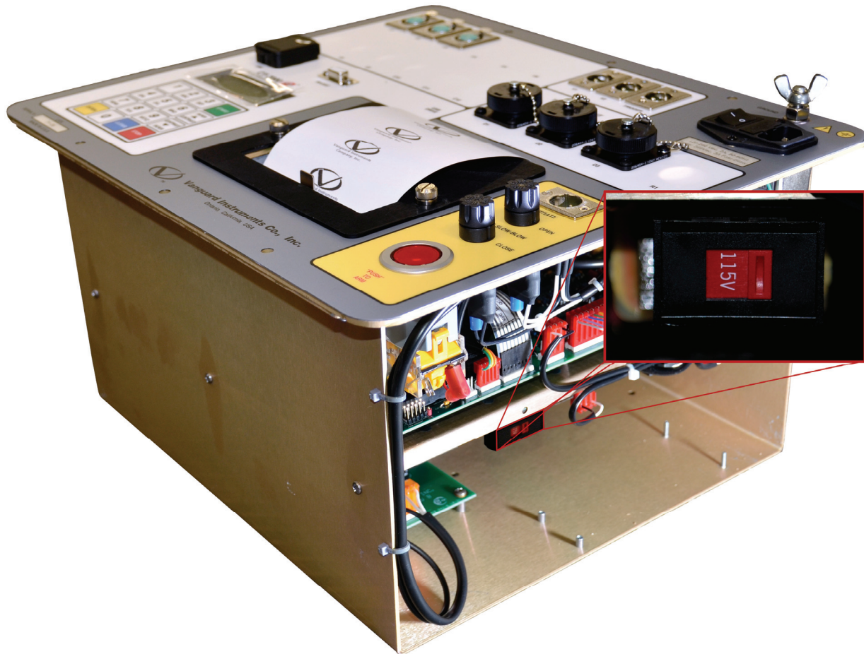
Figure 2. CT-7500 S2 Operating Voltage Setting Switch
