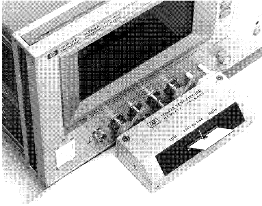
Figure 6-20. Connecting A Shorting Bar
