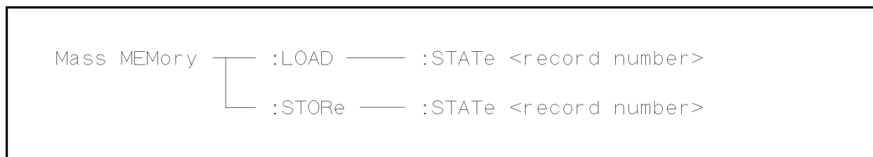
Figure 8-14. Mass MEMory Subsystem Command Tree
