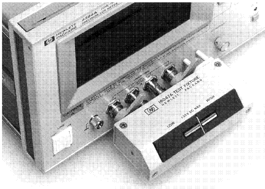
Figure 6-19. Connecting the 16047A
