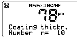
Figure 5.1: Display with Measurement (taken with the eddy current channel of a dual probe)
