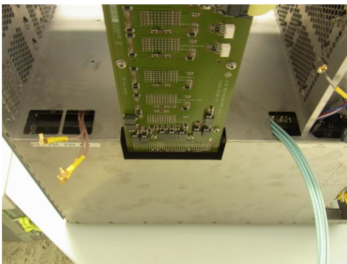
Figure 3-30: Cable routing with option R&S FSW-B71 installed
