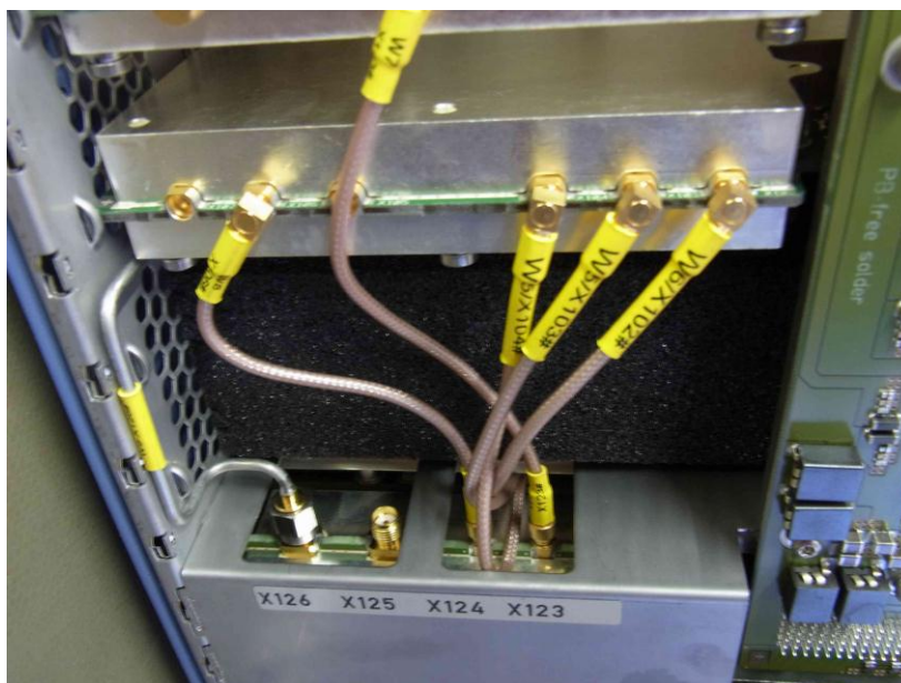
Figure 3-10: Cable routing without option R&S FSW-B71 installed
