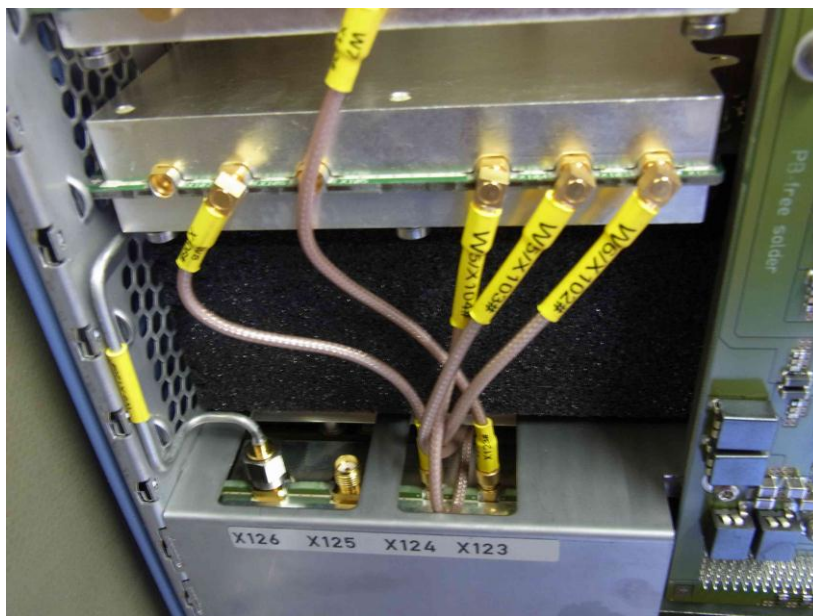
Figure 3-29: Cable routing without option R&S FSW-B71 installed
