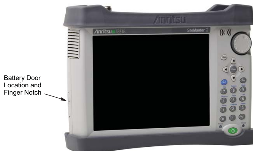
Figure 5-1. Battery Access Door Location and Finger Notch
