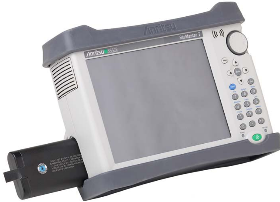
Figure 5-3. Removing the Battery
