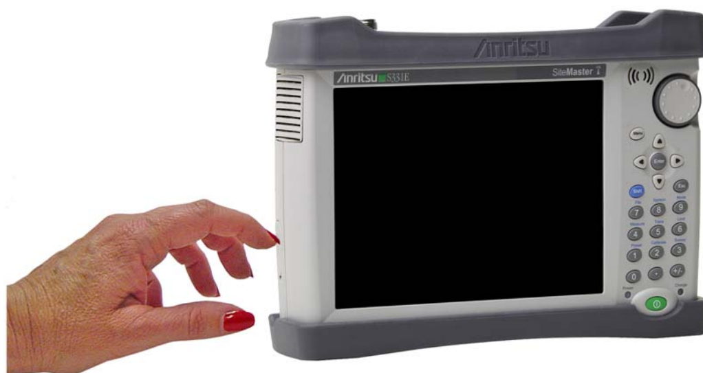
Figure 5-2. Opening the Battery Access Door
