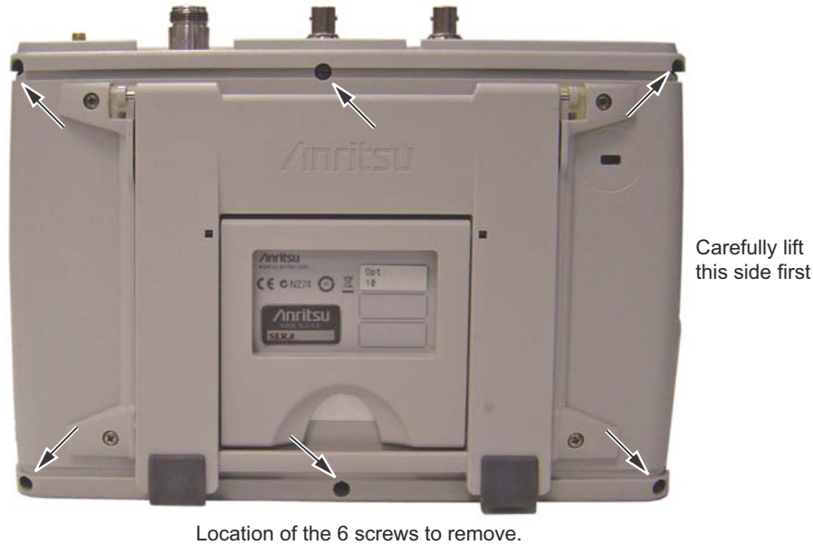
Figure 6-2. Remove the Four Screws
