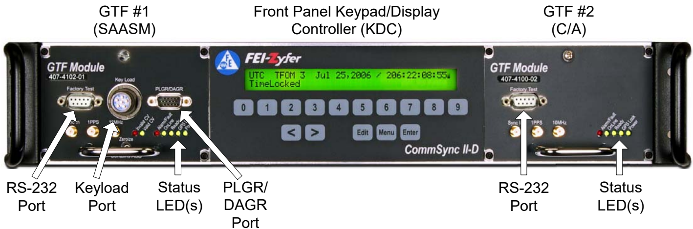
Figure 5-4 CommSync II-D Front Panel Port and Indicator Locations – GTF Systems
