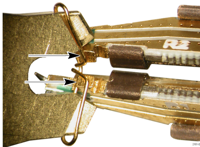
Figure 46: Set spring in front seat
