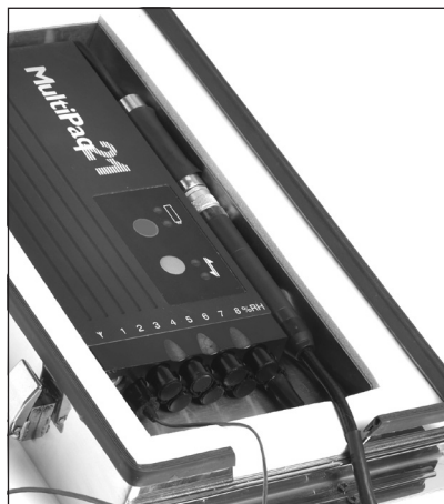
Sensor electronics in position in the thermal barrier's humidity-probe retainer.
