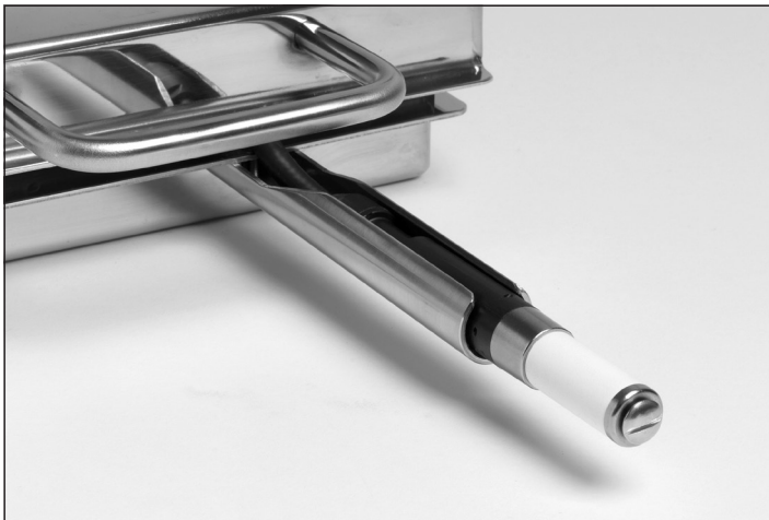
Humidity sensor positioned in a thermal barrier's mounting bracket. The sensor cap with PTFE filter is fitted.
