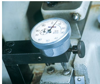
Displacement of can be read from above.
