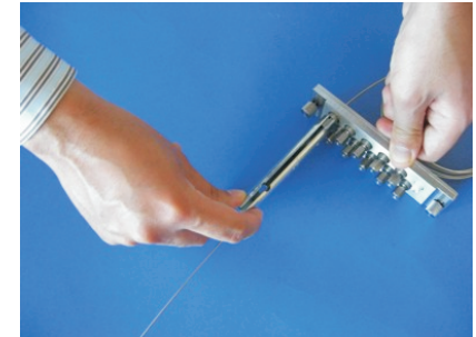
Using a bar or small screwdriver tighten the locknut a further 3/4 of a turn from the finger tight position. Do not overtighten.
