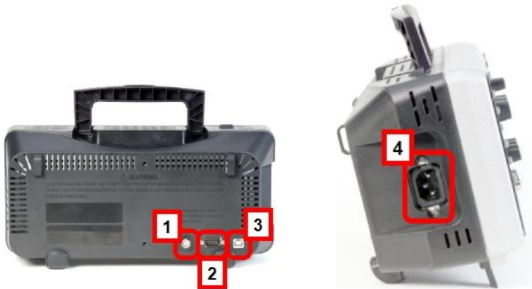
Figure 4-4. Back and Side panel connection locations on the 2 Channel WaveAce Oscilloscope.
