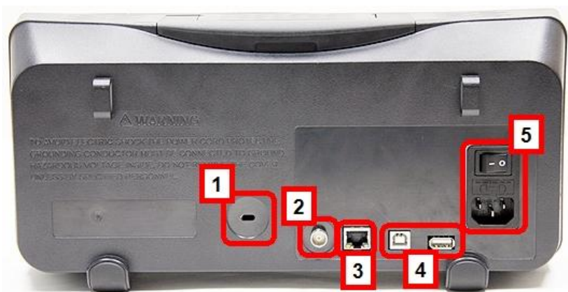
Figure 4-3. Back panel connection locations on the 4 Channel WaveAce Oscilloscope.
