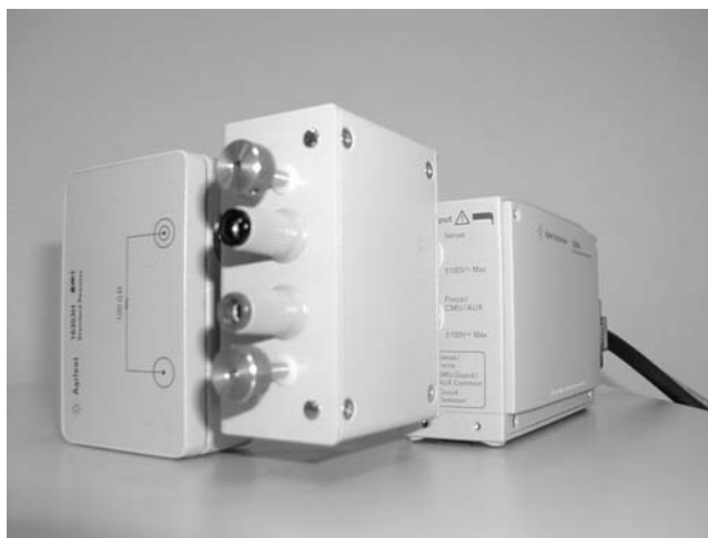
Figure 2-15 ASU connection for low current calibration adapter and calibration standard
