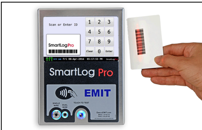
Figure 19. Using the barcode scanner
