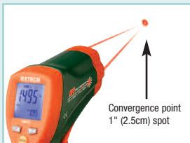
Two laser points converge at a distance of 30"/76.2cm (model 42512) and form a 1" (2.5cm) spot.
