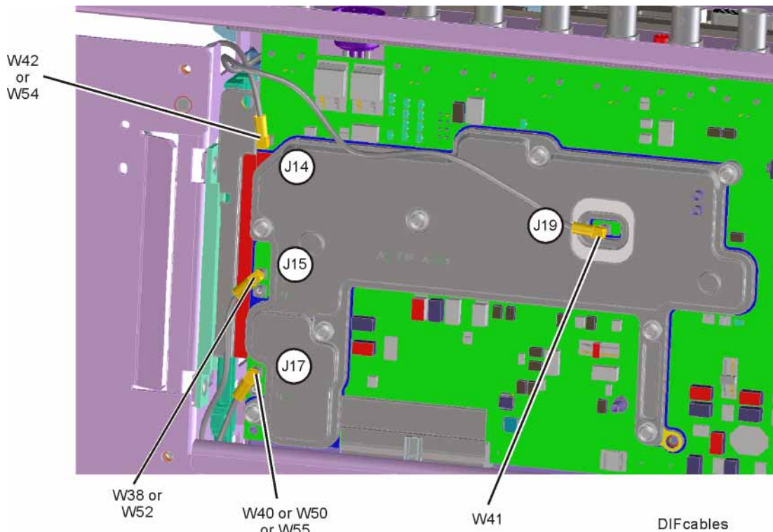
Figure 7-21 A3 Digital IF Cables
