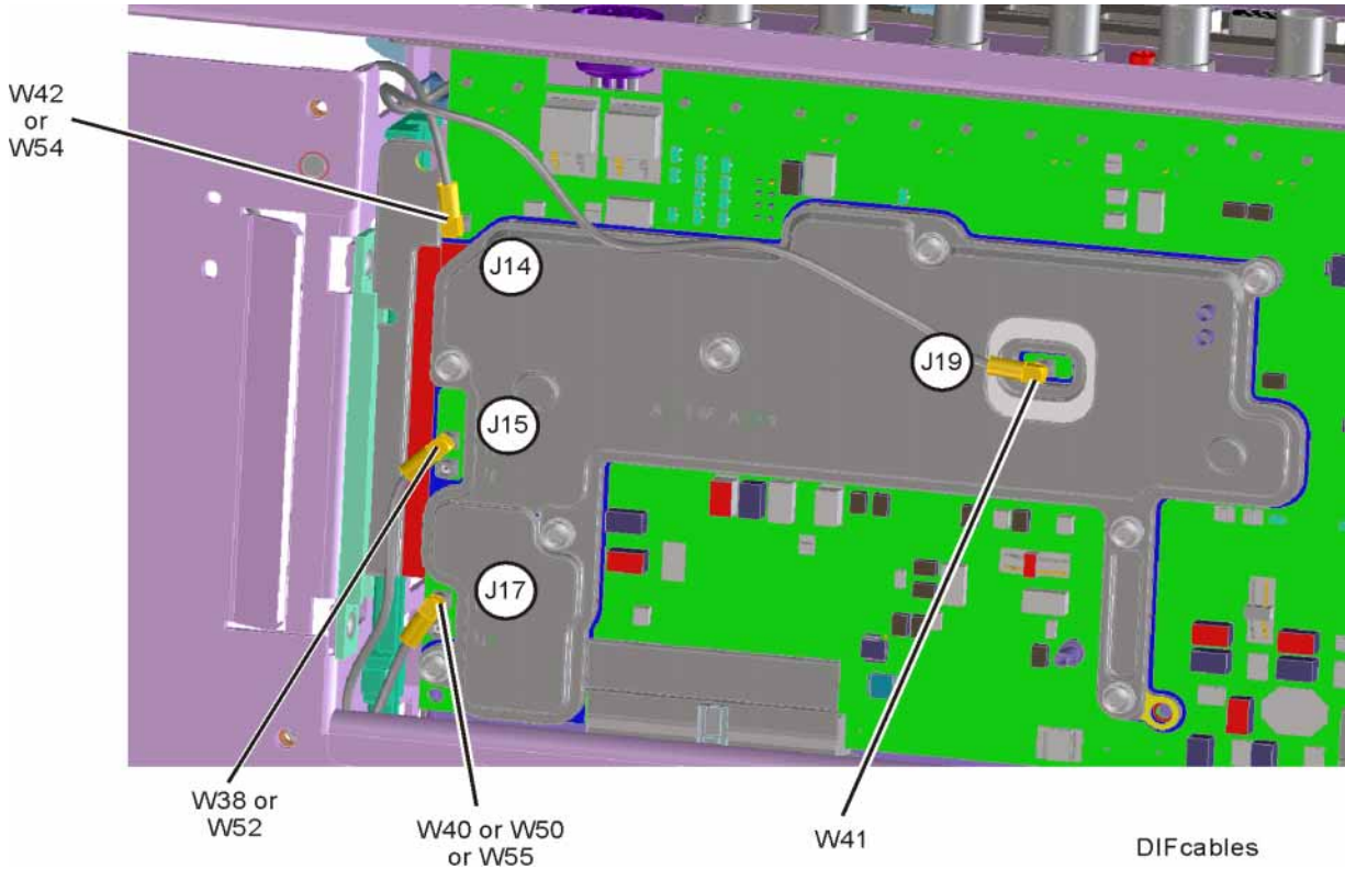
Figure 7-13 A3 Digital IF Cables
