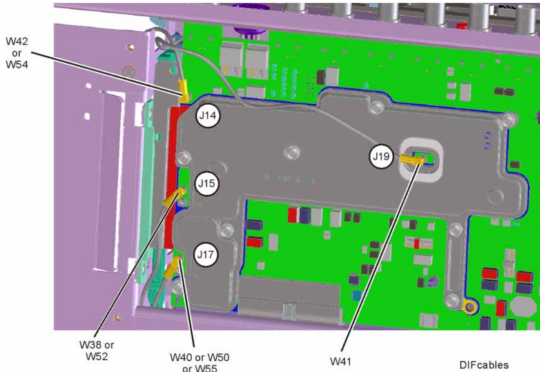
Figure 7-17 A3 Digital IF Cables
