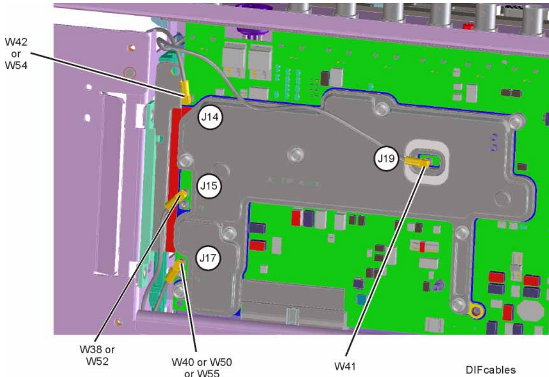
Figure 7-19 A3 Digital IF Cables
