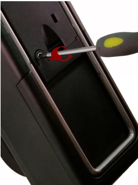
Step 1 - Remove security screw with Phillips screwdriver
