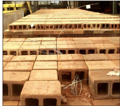
Thermocouples feeding through refractory bricks on the base of the kiln car to the thermal barrier below.
