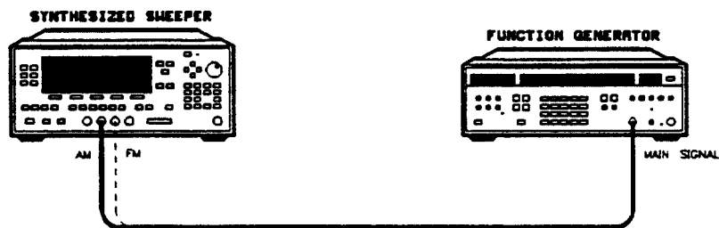
Figure 2-32. Modulation Meter Test Setup
