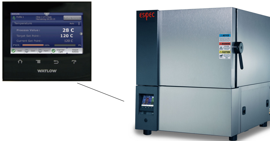
FIGURE 4.3. INSTRUMENTATION PANEL WITH WATLOW F4T CONTROLLER
