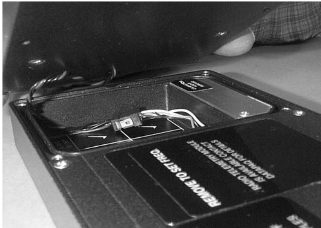
Expansion Paq (above) being fitted to Datapaq11, showing battery cables connected.
