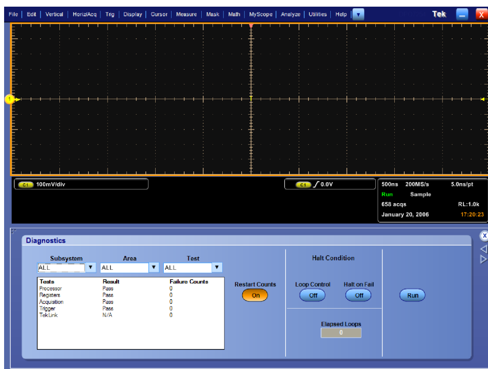
Figure 4-7: Diagnostics control panel
