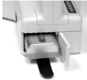
Figure 2-5 Prepare to insert the battery
