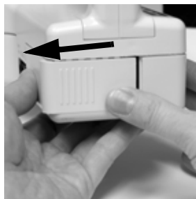
Figure 2-10 Unlatch Battery Compartment door
