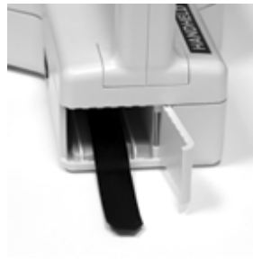
Figure 2-4 Pull Battery release ribbon out
