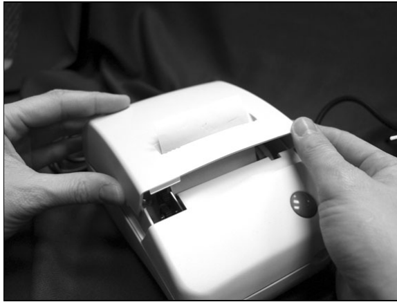
Figure 2-23 Feed paper through the printer's cover
