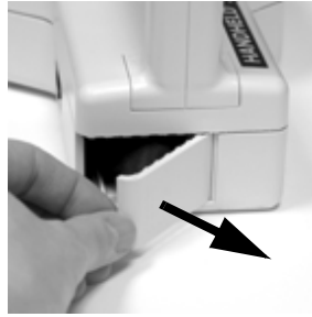
Figure 2-11 Open Battery Compartment door
