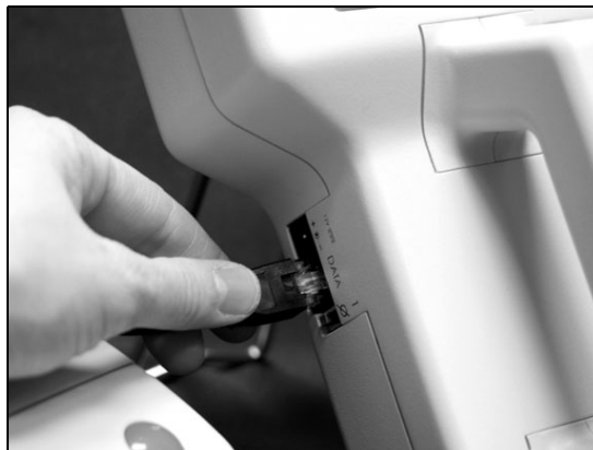
Figure 2-14 Attach printer cable to DATA port
