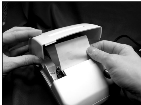
Figure 2-22 Preparing to feed paper through cover
