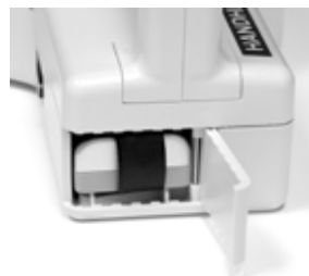
Figure 2-7 Tuck battery release ribbon
