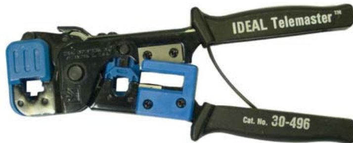
Figure 3-6 Typical RJ45 Crimp Tool
