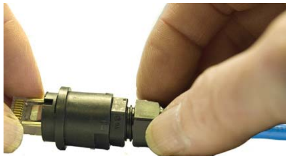
Figure 3-10 Tighten Cable Clamp Nut
