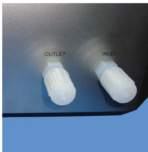
Figure 3-13 NC30+ Front Connections
