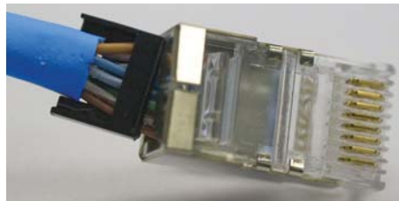
Figure 3-5 Loomed Wires Being Inserted into RJ45
