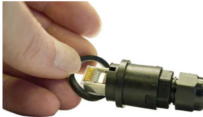
Figure 3-11 Install Connector Seal
