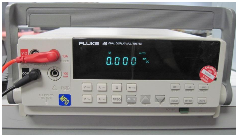
6.16. When you see the prompt “Far Left Section: Connect Ammeter to IDD_CAL_TP1 and IDD_CAL_TP2.” , then configure the Fluke 45 to measure current on the 10A range. See Photo 4 below.
