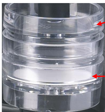
Figure 7-10: Gravimetric cassette and filter paper maintenance
