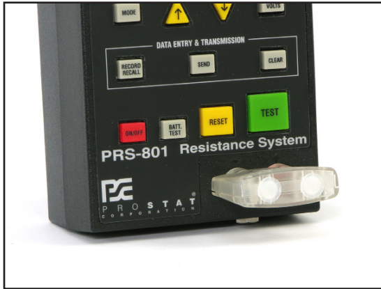
Figure 5: Low Resistance Range Calibration Shunt Installation
