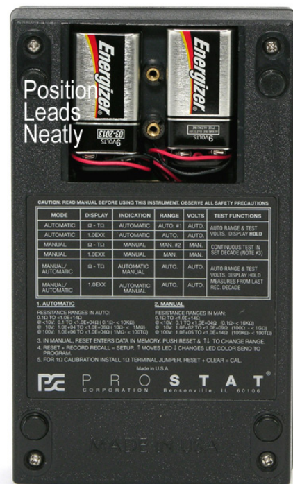
Figure 4: Install 2 each 9V Alkaline Batteries
