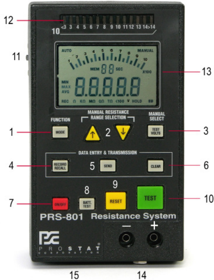
Figure 2: PRS-801 Controls & Display Indicators
