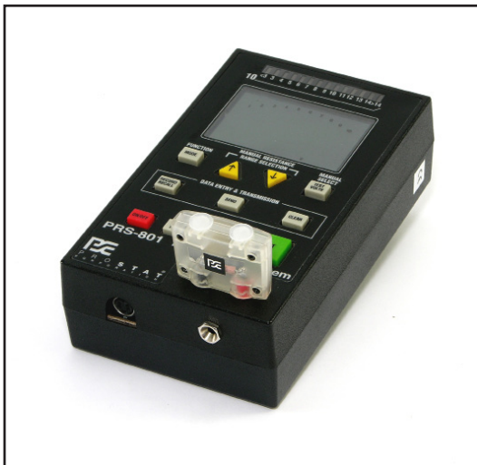
Figure 6: Low Resistance Range Calibration using Reference Module
