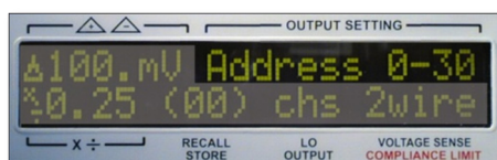
Figure 2.32 – Illegal GPIB Address Entry Display
