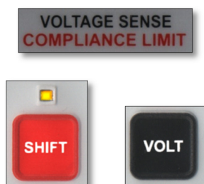
Figure 2.14 – Compliance Limit Setting Keys
