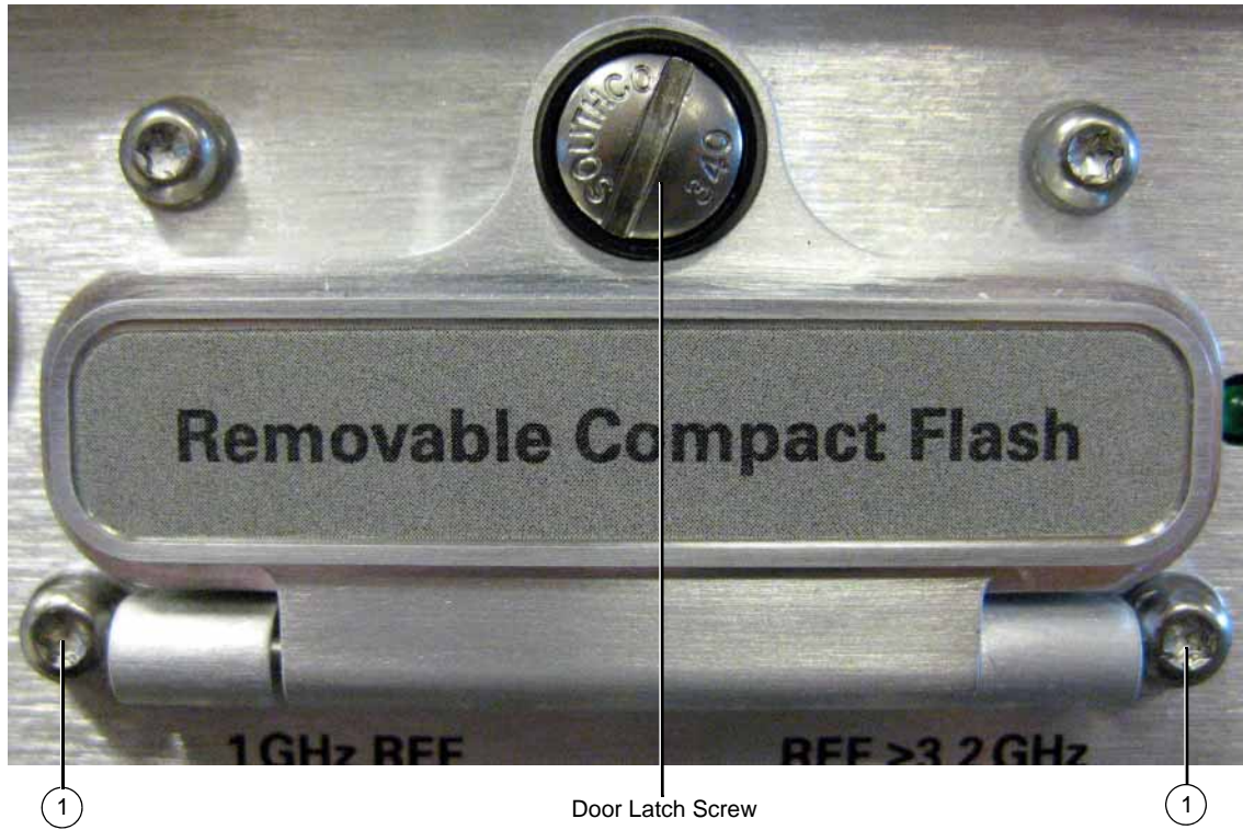
Figure 3-68 A41 Flash Drive Door Assembly
