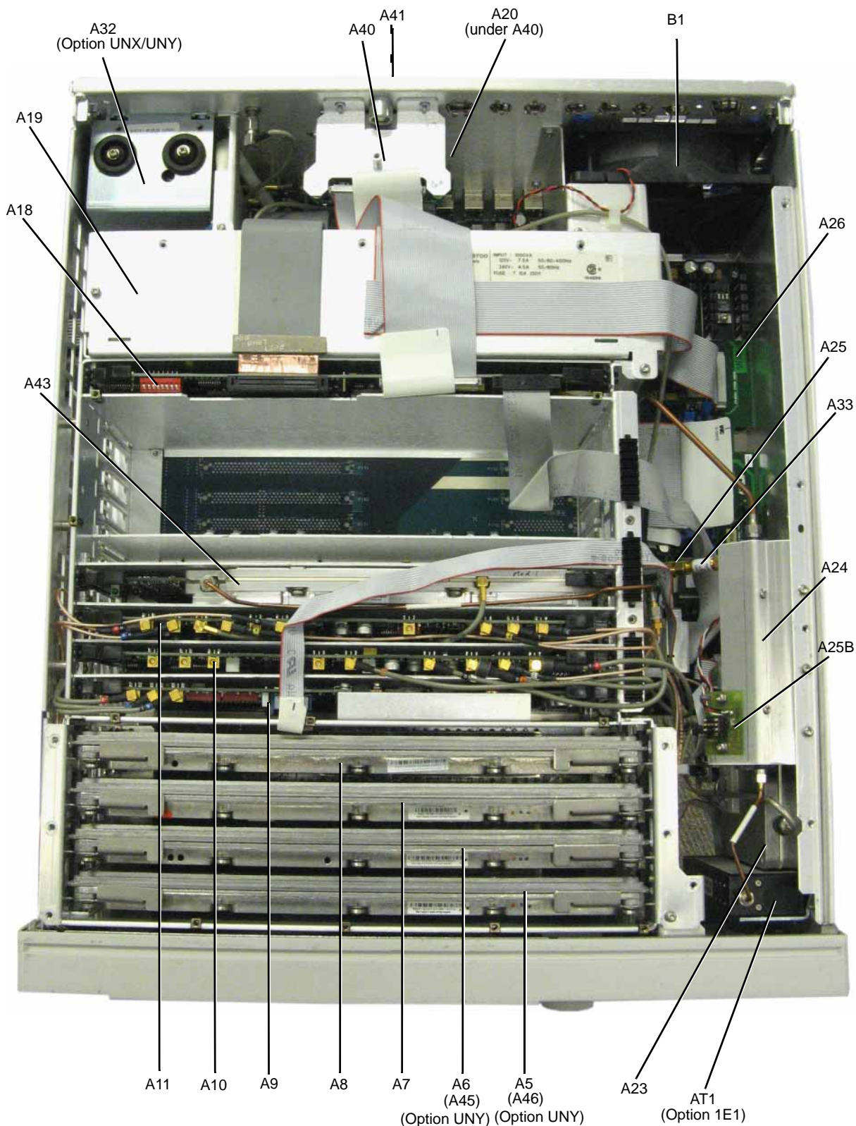
Figure 2-4 Assemblies from a Top View (E8257D Option 521)
