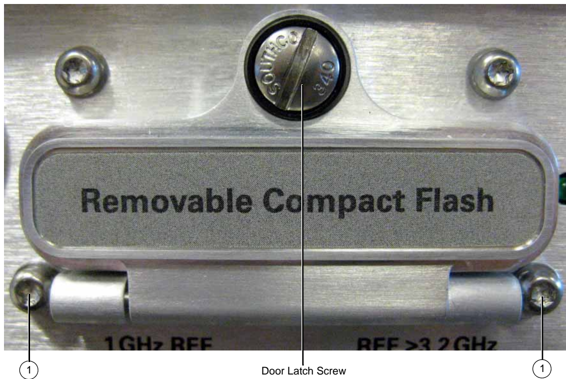
Figure 3-67 A41 Flash Drive Door Assembly
