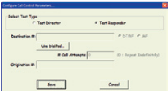
Figure 110 In the Configure Call Parameters window select Test Director or Test Responder. Default is test responder. Click save.
