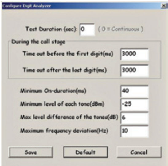
Figure 109 In the Configure Digit Analyzer screen set test duration, set time-outs before and after digits. Then set the minimum on-duration in milliseconds. The dBm level of each tone, the db difference level and finally the maximum frequency deviation in Hz. Click save. There is also a default setting available.
