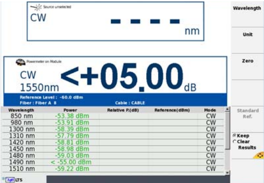
Figure 111 Results and commands of the power meter
