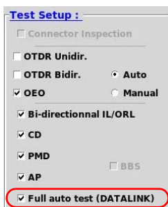
Figure 244 Test sequence configuration on 8000 V2
