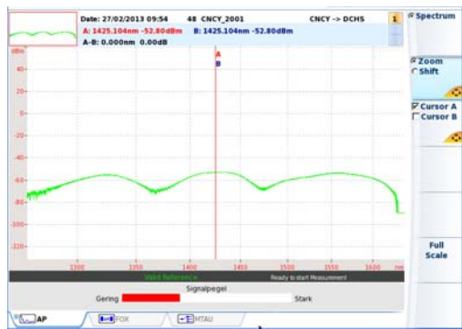
Figure 203 Example of a reference for a broadband source
