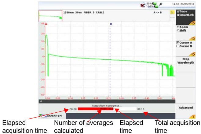
Figure 31 Acquisition in progress with Expert OTDR
