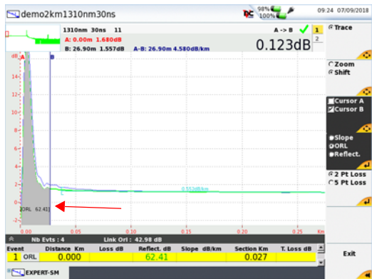
Figure 51 Result of ORL measurement
