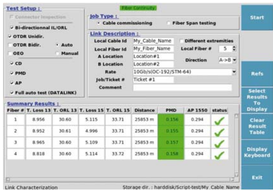
Figure 251 Fiber Characterization Results Table
