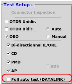
Figure 248 Test sequence configuration on 8000 V2
