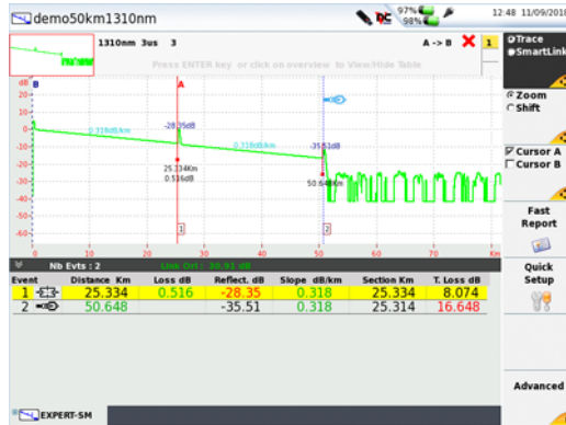
Figure 38 Example of trace and results table in Expert OTDR
