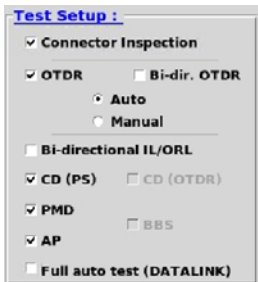
Figure 240 Test sequence configuration on 8000 V2
