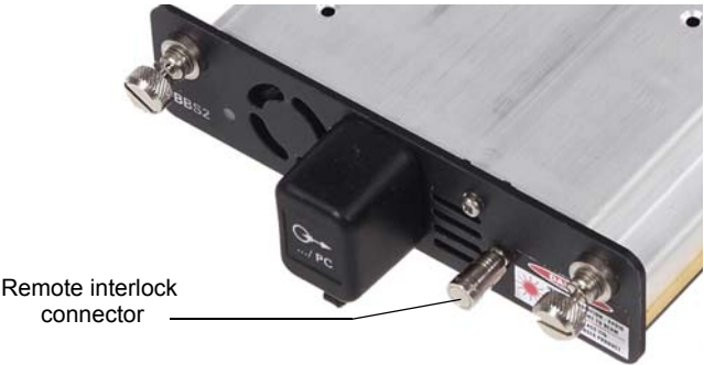
Figure 224 Remote interlock connector
