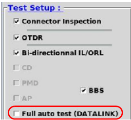
Figure 249 Test sequence configuration on 6000A
