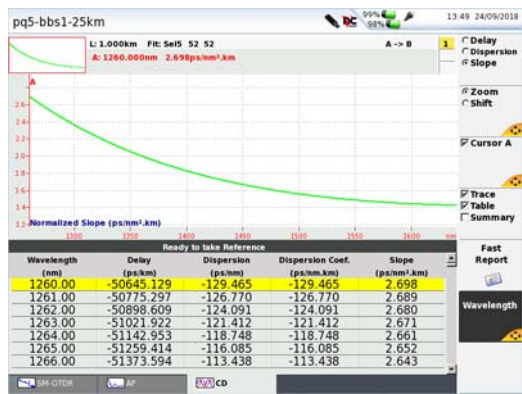
Figure 216 Example of the Slope display
