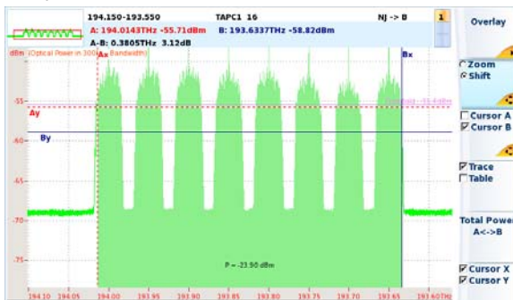
Figure 196 Display of total power between the cursors
