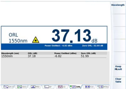
Figure 266 Results for an ORL manual measurement
