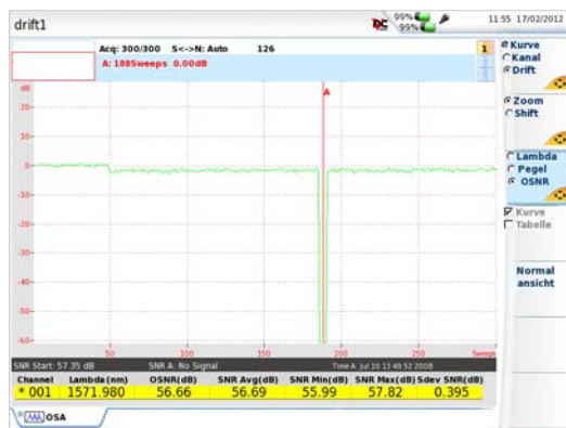
Figure 148 Example of drift measurement, wavelength over time
