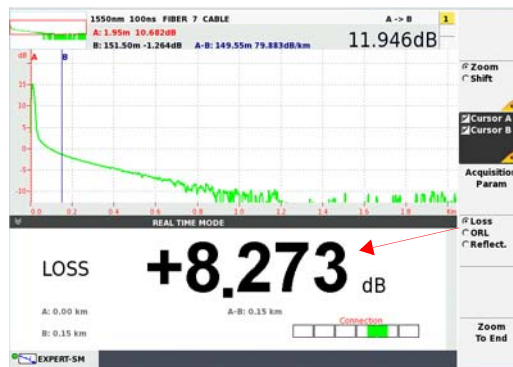
Figure 34 Example of loss measurement
