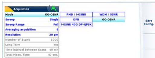
Figure 198 OSA Setup: OO-OSNR configuration
