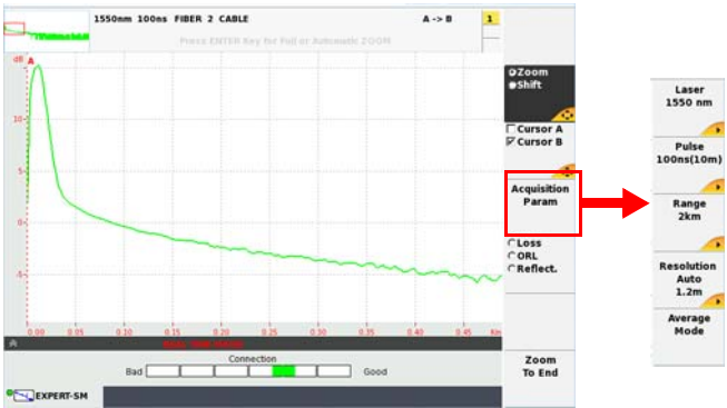
Figure 33 Example of acquisition in Real Time
