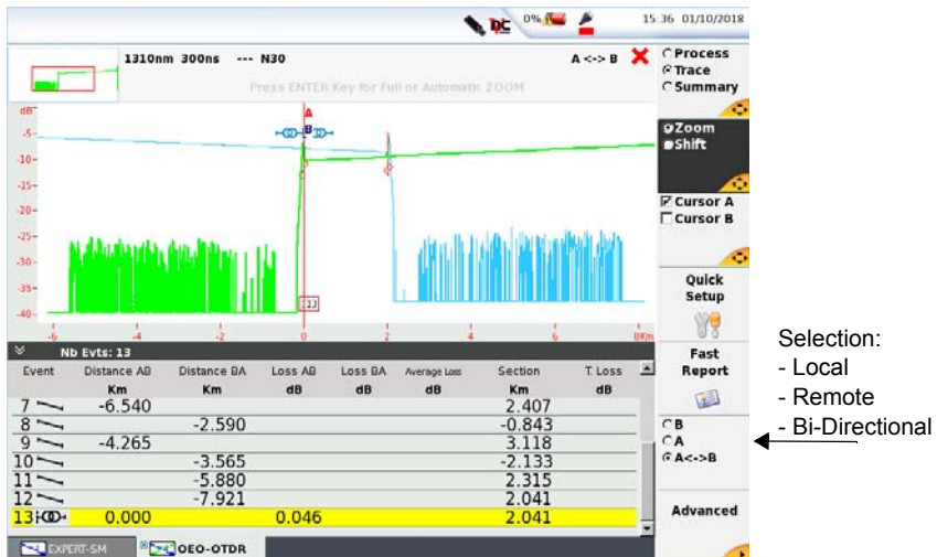
Figure 118 Butterfly representation of the bi-directional measurement
