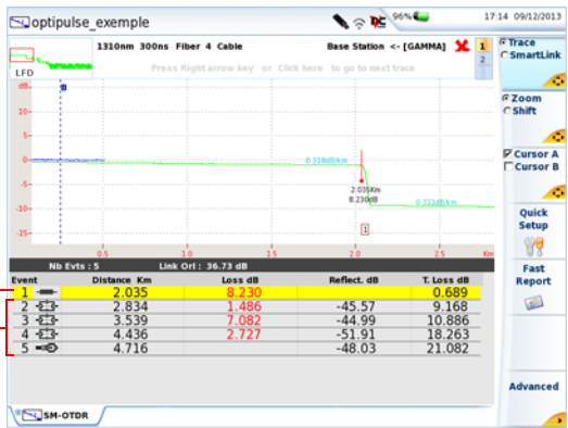
Figure 67 OTDR Traces with OptiPulses
