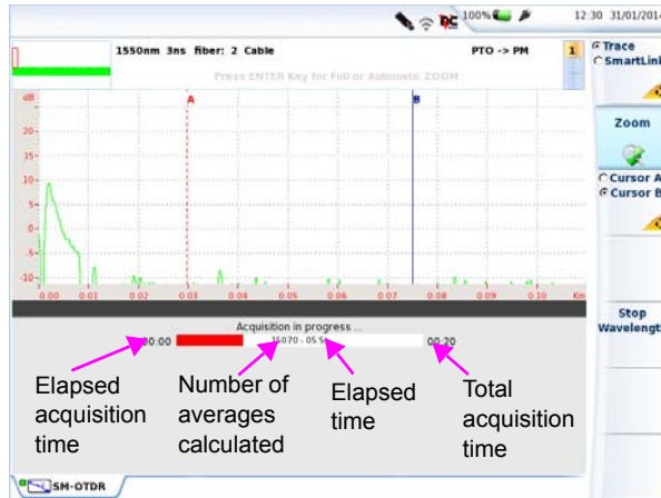
Figure 73 Acquisition in progress
