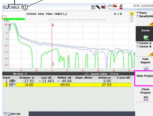
Figure 63 Trace from fiber selected in project Name of the label Number of the fiber tested
