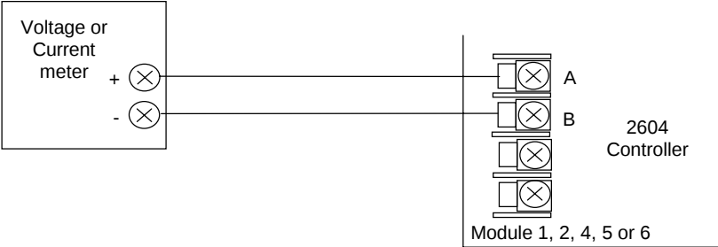
Figure 24-4: DC Module Connections Volts or Current Output
