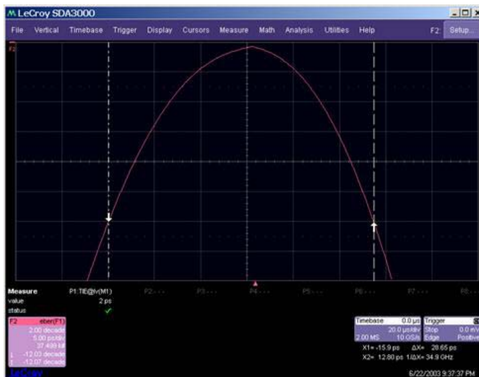
Figure 5-39. Total jitter curve. The vertical values of this curve represent the probability of a data transition occurring at a time represented by the horizontal axis. The horizontal center of the plot is 0 ps. The two markers are placed at the vertical level corresponding to a bit error rate of 10 \times 10^{-12} and the horizontal distance between these two points is the total jitter at this bit error rate.
