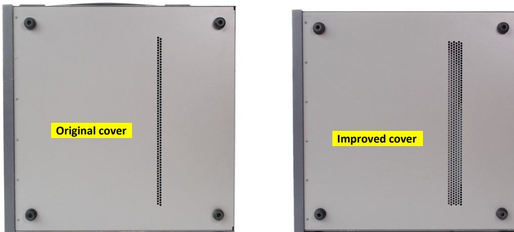
Figure 2 APx586 original (left) and improved (right) covers
