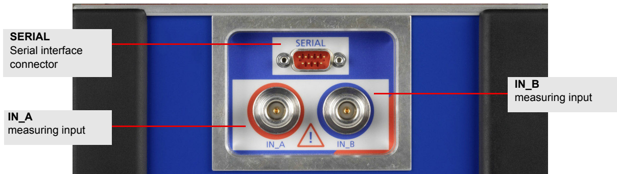
Figure 3-4: Right side view of the CP TD1
