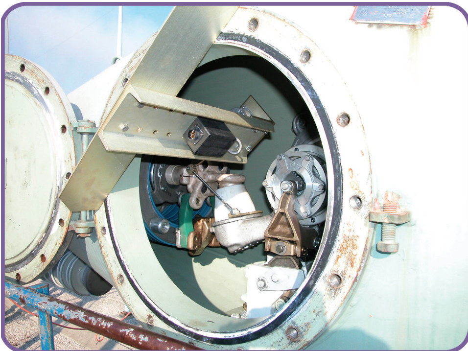
Figure 29. Westinghouse SFA Transducer Installation
