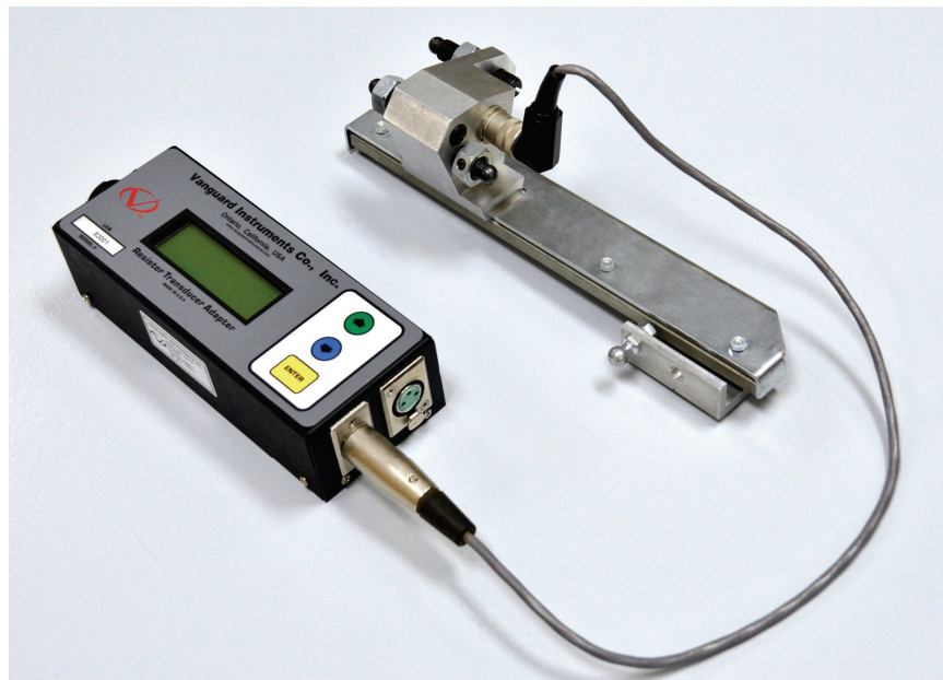
Figure 11. Vanguard Resistor Transducer Adapter Connected to an ABB AHMB Transducer
