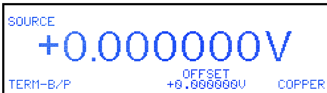
Figure 11-1: Initial Operating Screen for Voltage Tests
