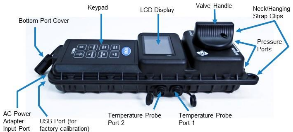
Figure 1-1 HM675 Meter Description
