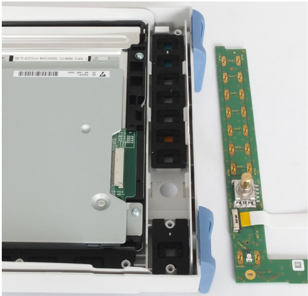
Figure 4-9: Silicone Keypads under the Key PCB
