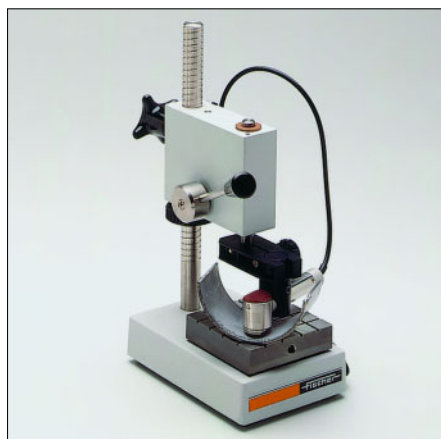
The angle probe Z11NG in combination with support stand V12 used to measure the coating thickness in bushings, pipes, bearing shells, etc. with diameters of 32 mm (1 1/4") and up.
