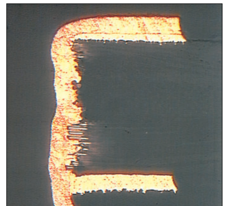
It clearly shows that the voids, which are result of fibers torn by drilling, were subsequently metallized. This effect also makes optical determination of the copper thickness more difficult.
