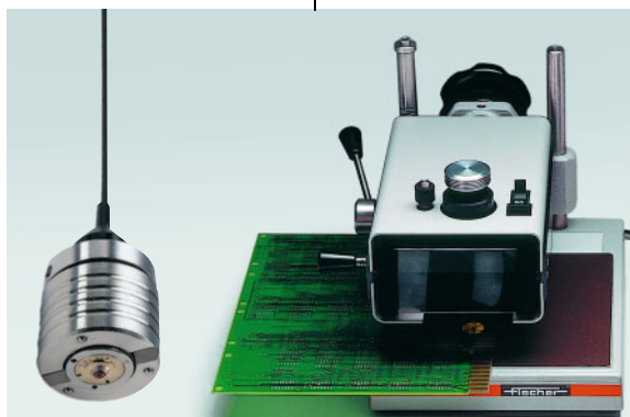
... coating thickness measurement according to the Beta backscatter method
