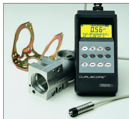
DUALSCOPE® MP40E with probe ED10 to measure coating thickness on ferromagnetic, as well as non-ferromagnetic materials with automatic recognition and selection of the measurement method.
