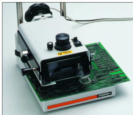
Measurement with the universal measurement stage Z6NG using isotope PM147 and aperture ring ø 0.63 mm (ø 0.02").
