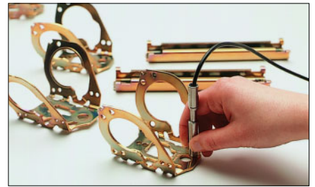
Measurement of zinc coatings.
