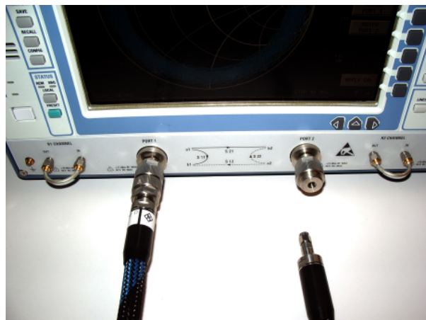
Figure 1-7: Network analyzer setup for calibration
