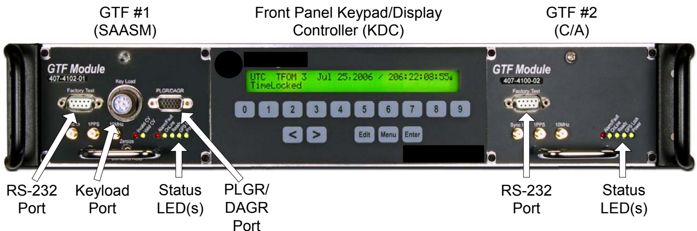
Figure 5-4 SyncPort 64 Front Panel Port and Indicator Locations – GTF Systems
