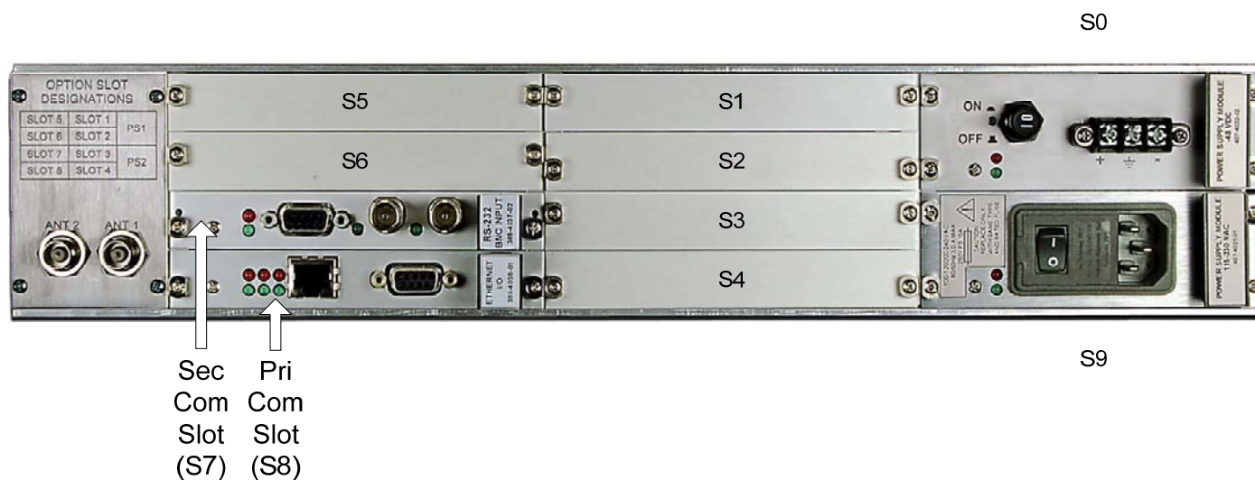
Figure 4-4 SyncPort 64 Rear View – With Communication Modules
