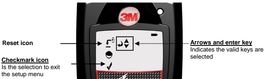
Figure 4-6: Resetting the Edge from the keypad
