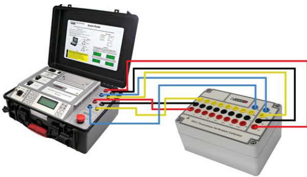
Connecting TRT with 4 connectors for H cables and 4 connectors for X cables
