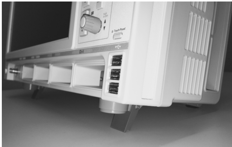
Tilting up the Front of the CX3300
