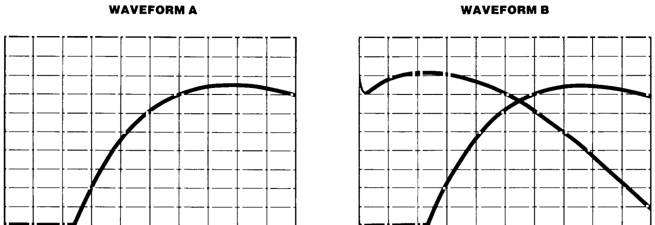
Figure 5-25. Spectrum Analyzer Waveforms of YO Loop Gain
