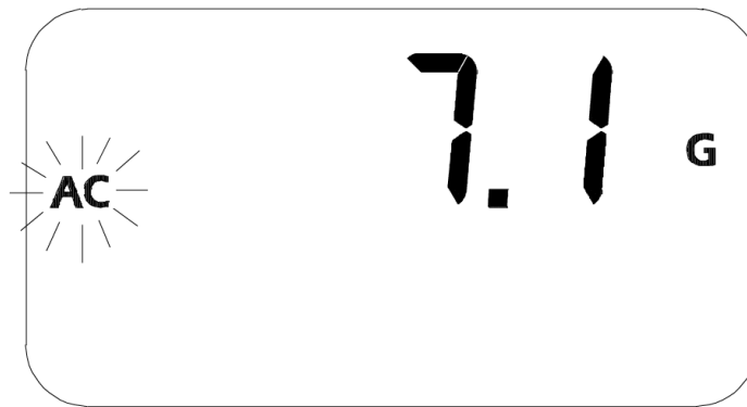
Figure 3-19 Low AC Signal Indication
